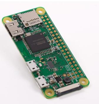
The low-profile (2.6" x 1.2" x 0.2") Pi Zero technically has a full-size GPIO header, but the pins have to be soldered on by the user if they are needed.
