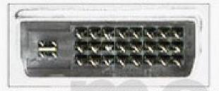
Three rows of 8 pins and two contacts above and below the flat blade
